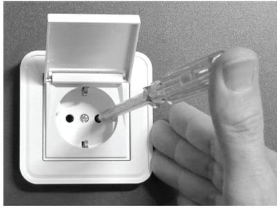
→ In this way, you can quickly determine the opening of phase L, for example in a power socket.
