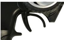
2. Slowly pull the throttle/brake lever towards the handle to make the vehicle move forwards.
