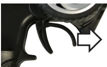
→ Do not switch immediately between forwards/reverse. Bring the vehicle to a standstill first before moving it in the other direction. Directly switching to another direction may overload the drive components.
