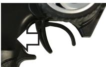
3. Slowly push the throttle/brake lever away from the handle to make the vehicle move backwards.
