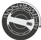
Low Z voltage measurement
