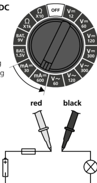
**!** No currents above 600 mA may be measured in the mA range. Currents above this level trigger the automatic fuse in the meter (F 630 mA / 300 V, Ø 5 mm x 20 mm).
