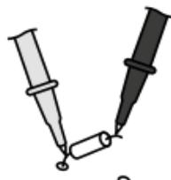
Resistances can only be measured correctly in isolation; therefore, the components might need to be disconnected from the remainder of the circuit.
