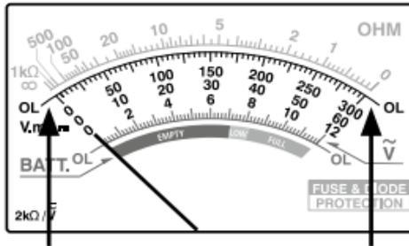
If the pointer remains to the left of the "0" during the measurement or to the right of the "0" when measuring resistance, either the test prods are mixed up or the measuring circuit is interrupted. Repeat the measurement with the test prods changed over.
