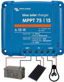
Figure 4: Power connections
