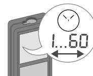
Once the key is released with the laser activated, the remaining seconds until the measurement are displayed in a countdown. The delayed release is recommended for precise aiming e.g. at long distances. It avoids shaking of the device when pressing the measurement key.
