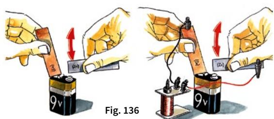
A magnetic field forms around the coil in such circumstances but as soon as the circuit is opened the magnetic field is destroyed, the consequence being an induced current that is felt as a shock.
