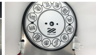
The installation of the scan backboard is completed.
