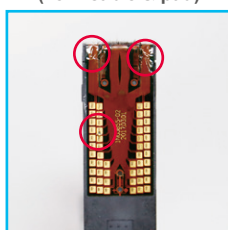
NG Cartridge (Torn cable & pad)
