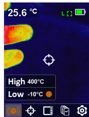
The temperature alarm ranges correspond to the temperature alarm setting menu.
