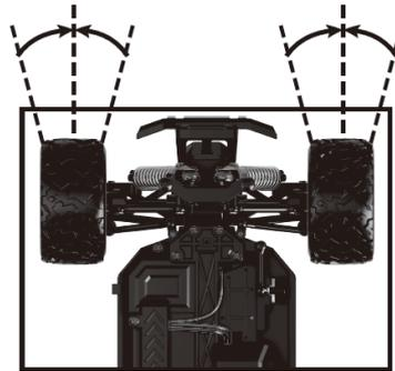
Gently pull the throttle trigger to allow the car to run slowly. In the meantime tune the steering trim until the front wheels keep aligned.
