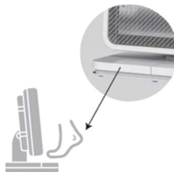
There are two heating elements controlled by foot switches.
