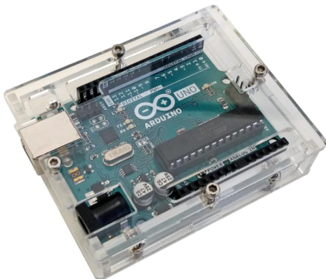
Use the short screws to secure the Arduino® board. Use the spacers to offset the board from the bottom.
