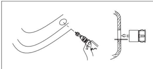
Drill the holes for the four ultrasound sensors with the enclosed 21 mm drill.
