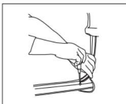
Attach the control unit with the enclosed adhesive pad. A suitable place is the side wall in the watertight trunk close to a taillight. Make sure that the connection lines of the sensors reach up to the sensor units.
