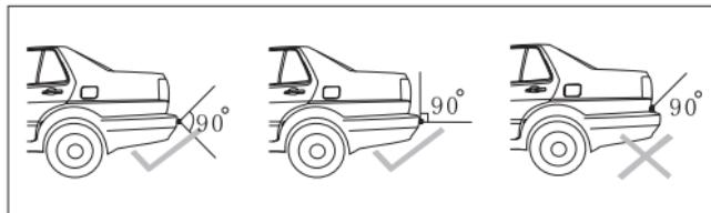
The ultrasound sensors must be installed evenly across the width of the vehicle.
