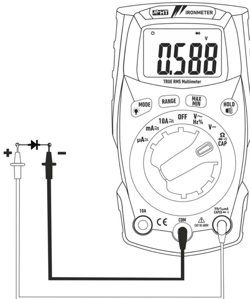
Fig. 6: Use of the instrument for diode test
