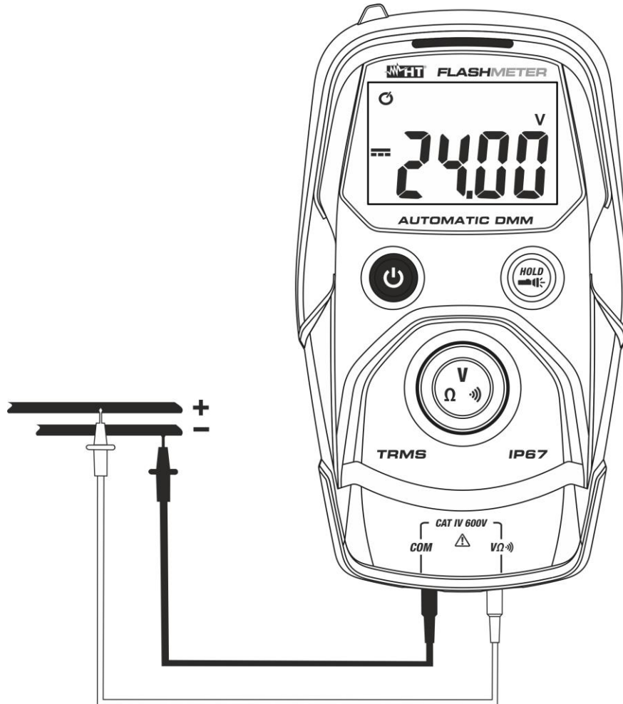
Fig. 3: Use of the instrument for DC voltage measurement
