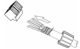
2. Put cable into IDC according terminal T568
