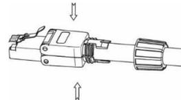
5. Press down both side metal housing until the wire into the IDC pin case.
