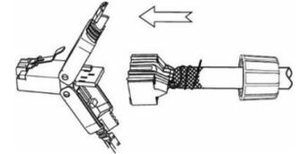
4. To insert IDC into PCB
