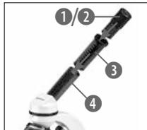
Now, insert the 10x eyepiece (1) into the Barlow lens (3). Make sure that the Barlow lens is placed all the way into the eyepiece supports (4) and is not pulled out.
