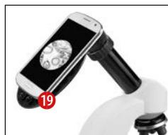
Attach the smartphone holder to the eyepiece.
