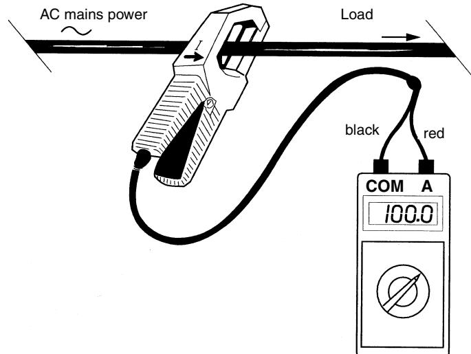
**⚠** From 500 A to 600 A, limit the current clamp operating time: 10 minutes on and 30 minutes off.
