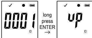
Press the button DOWN (5) several times until the 4 digit logger identifier and "ID" are shown on the display.
