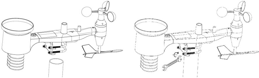
Use the "WEST" indicator to make sure the sensor is facing the correct direction.
