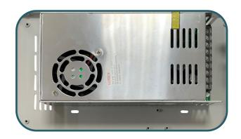
5. Now, screw the fan control next to the Power Supply with the remaining black screws and connect the fan to the connector provided for this purpose.
