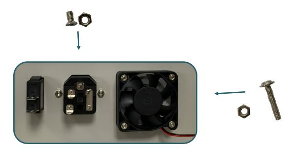
4. Now, mount the power supply into the case. Therefore, you have to screw it from the bottom of the case with the big silver screws.
