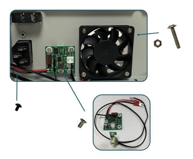
3. Now, mount the power supply into the case. Therefore, you have to screw it from the bottom of the case with the big silver screws.
