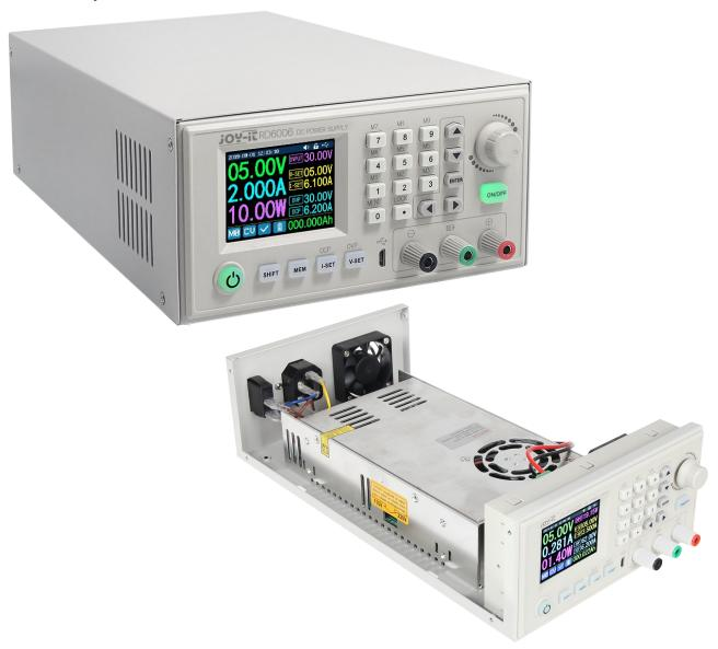
You can adjust the output voltage of the RD6006-NT with the help of the fine-tuning potentiometer. You can see your adjustment at the input voltage of your RD6006 / RD6006P. Ideally, the RD6006 / RD6006P has an input voltage of 65 V to be able to reach the complete 60 V.
