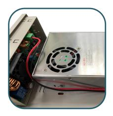
7. You can also connect the connector from the temperature sensor lead-out if you want to lead the temperature sensor outside of the case. Otherwise, connect the temperature sensor now to the RD6006 / RD6006P.
