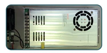
4. Now, connect the fan to the fan controller and the fan controller to the power supply. Therefore, connect the black cable of the fan control to the power supply with one of the anticipated terminals V- and the red cable with one of the V+ terminals.
