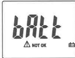
Fig. 2: Low battery indication
