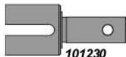
101230 Diff Shaft 5x23.5mm Differentialwelle 5x23.5mm Axe différentiel 5x23.5mm デフシャフト 5x23.5mm
