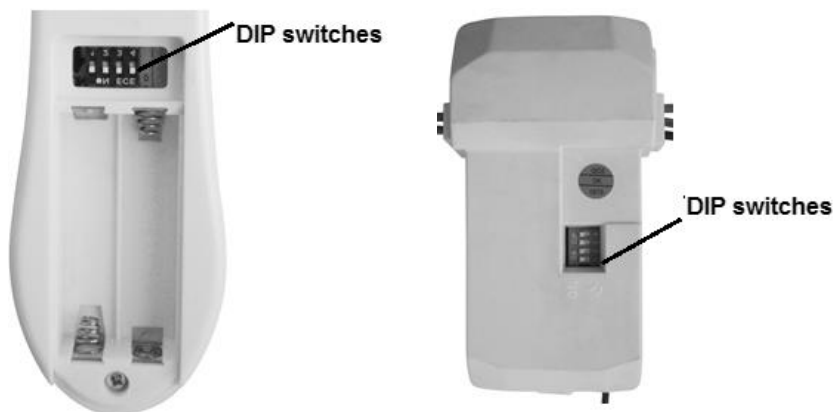
Fig. 8 Remote battery compartment
