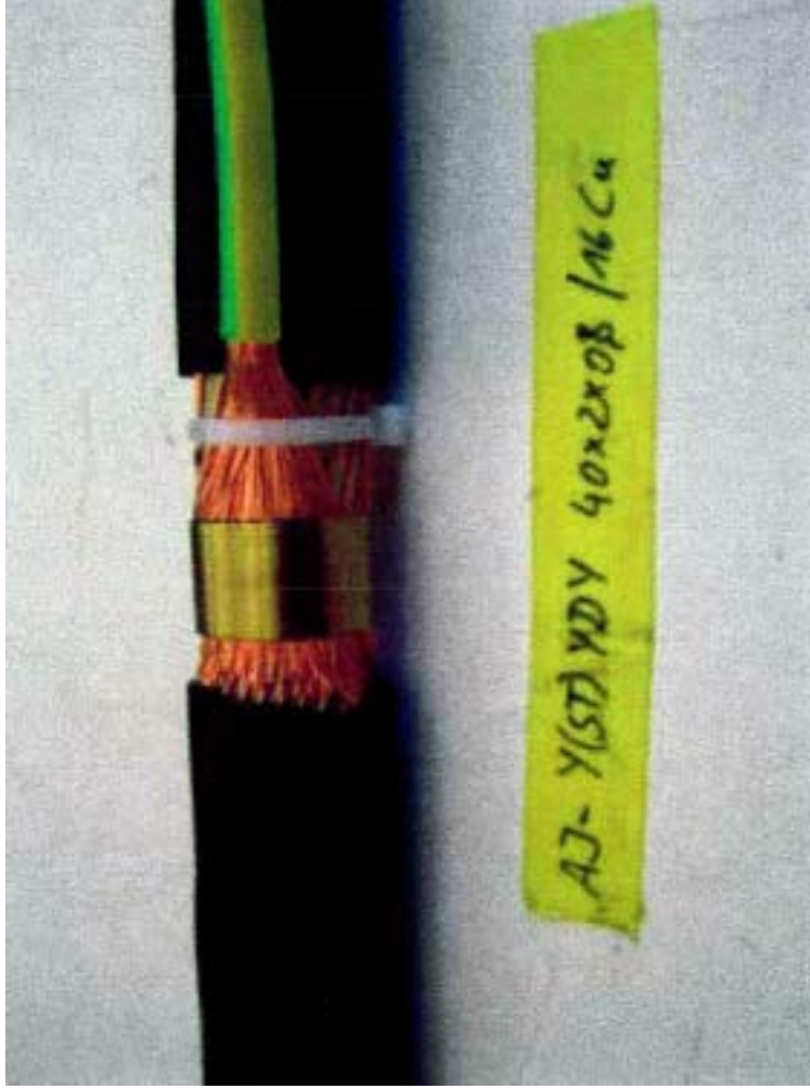
Fig. 2.4: Contact force spring complete mounted; for better stabilisation this could be fixed with a cable tie
