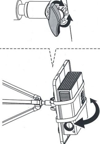
Loosen the round locking knob and rotate the tray to the proper position as shown, then tighten the round locking knob.
