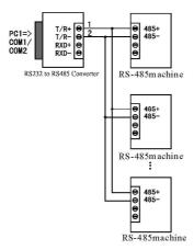
half-duplex communication connect between 3. interface converter
