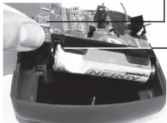
**2** Take off the upper part of the housing and lift the PCB slightly to reach the battery easily (b).
