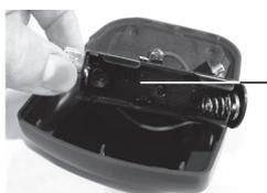
**3** Remove the battery and dispose it according to above mentioned regulations (c).
