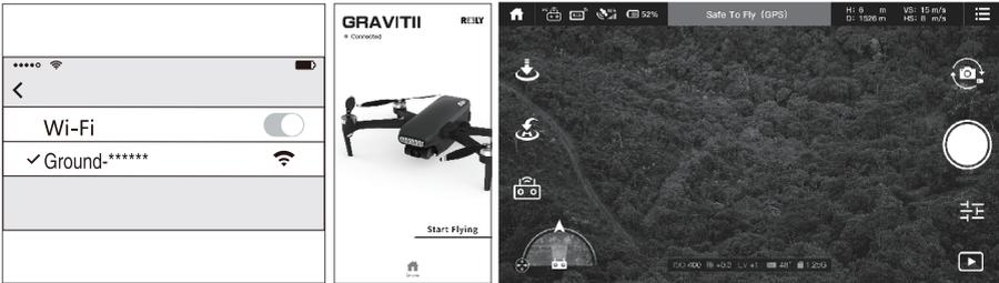
Open Graviti app to check whether the drone status in the upper left corner is connected. If "connected " is displayed, click "start flying" to enter operation interface.
