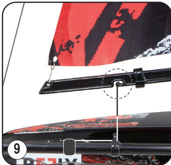
Attach the chord loop to the jib boom hook.
