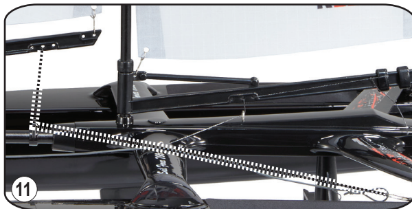
Thread the jib boom cord through the eyelets and attach the loop to the pin.
