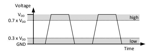
Figure 4: SDA and SCL logic levels
