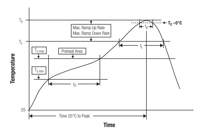
Figure 13: Reflow soldering profile
