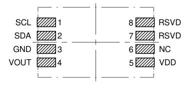
Figure 2: Pin specifications (top view)
