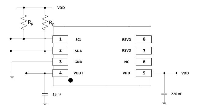
Figure 8: Application circuit with I<sup>2</sup>C interface (top view)
