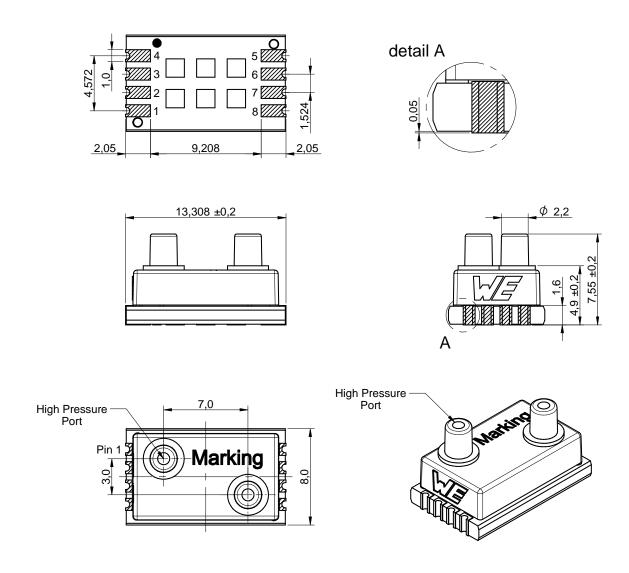
Figure 10: Sensor dimensions [mm]
