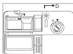
If the corresponding message does not light up in the display, you can estimate the amount of remaining rinse aid to the optical level indicator (D) next to the dispenser.
