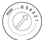
Take off the lid of the rinse aid dispenser and adjust the dial to the desired level. The factory setting is "4".
