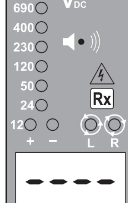
Ensure the circuit under test is not energised. Connect both test probes to the circuit. The continuity LED illuminates and buzzer sounds continuously to indicate continuity  $< 500 \text{ k}\Omega$ . Note: No continuity measurement is available on the LCD display.
