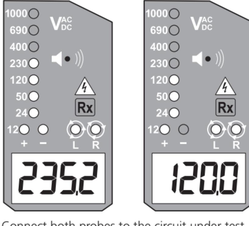
Connect both probes to the circuit under test. The voltage is indicated by LEDs and the LCD display.
