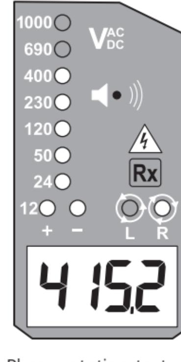
L LED and R LED's for the Phase rotation test may operate on various wiring systems, but an effective test result can only be obtained on three-phase 4-wire systems.
