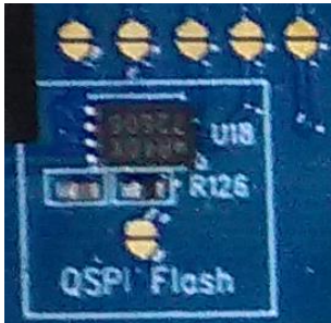
Figure 18: Optional external serial SPI flash IC (U18) schematic and PCB
