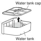
\*Please drain water from diagonal position of the water tank's handle.(as shown)
