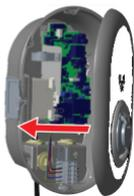
5. Switch the charging station on. The previously stored Master and user RFID cards are deleted.
