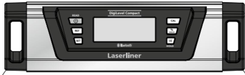
3. Now turn the unit around horizontally (end-for-end) by 180° such that its ends are positioned opposite where they previously were but again exactly at the underlying surface marks (reverse measurement). Then press the READ button (1) again. -2- flashes. The subsequent acoustic signal concludes the process.
