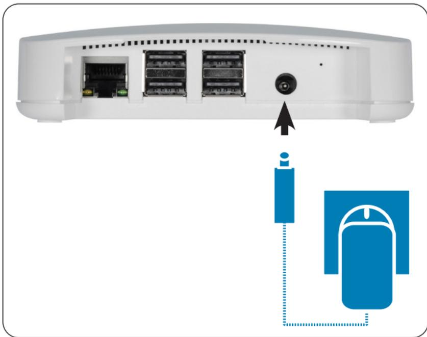
After switching on the power supply, the LED starts to flash green and the red LED flashes during the boot process.
