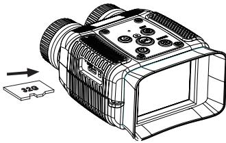
Open the protective rubber cover on the side of the device and push the memory card into the card slot until it locks in place. To remove the card, push it in slightly until ejected.
