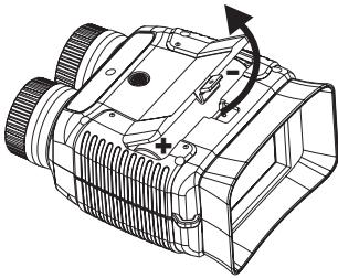
Open the protective rubber cover on the side of the device and connect the included USB-C™ cable to the USB-C™ socket. Connect the USB-A plug to a computer or a USB charger.
