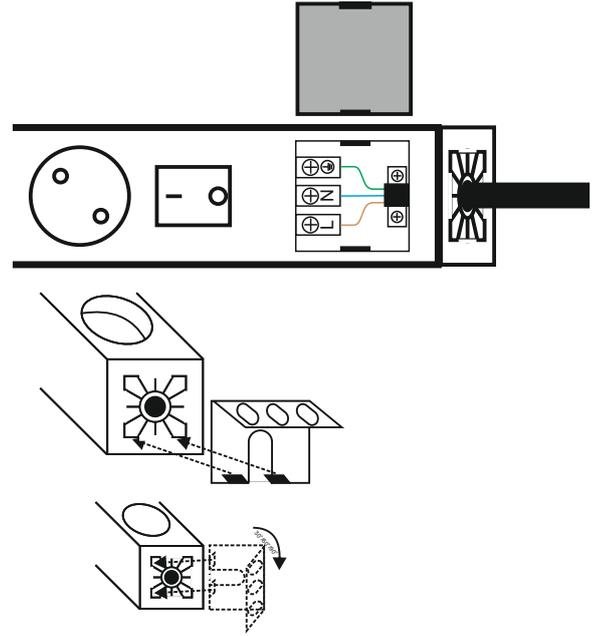
To mount it in the server cabinet, insert the retaining lugs of the Brackets in the side slots.
