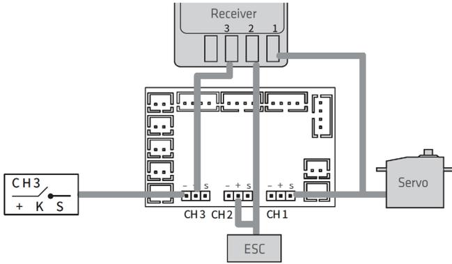
**CH1:** Both ends of the wiring harness are connected to the servo or CH1 of the main control board.
