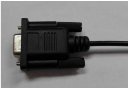
DB9 to computer serial port
