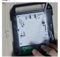
Unscrew 4x light source board screws.
