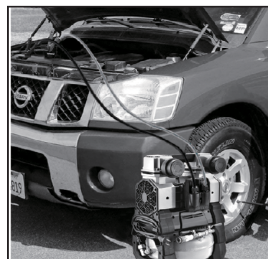
Battery via leads (DC)
