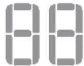
**Humidity and Timer display** – When the appliance is turned on, it displays the current humidity level in the room. When the humidity level is adjusted, the selected humidity will blink shortly on the display then current humidity level be shown.
