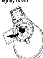
4. Fit the worm-drive housing with the pulp outlet facing left and the juice outlet facing forward to the drive unit.
