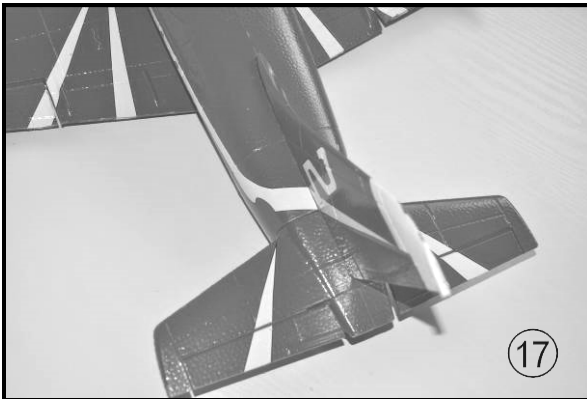
Fig. 17 - Glue the vertical stabilizer as shown in the photo (glue not included).
