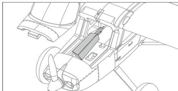
1. Before connecting the battery to the plane, power on the transmitter and ensure throttle lever in the lowest position.
