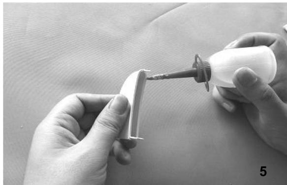
**Fig. 5 -** Glue the servo fairing.
